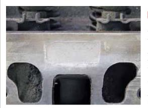
Removing the masks and tape revealed that the cement-filled opening was in fact completely flush with the intake flange. If a depression exists, the only real recourse is to chip the cement away with a hammer and screwdriver and start over again. (In either instance, be sure to carefully mask accordingly to keep contaminants out of the engine.)
