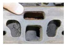
Beginning in '72, Pontiac added this hole above the exhaust crossover. Said to keep oil flowing under the valve cover isolated from exhaust heat, it's completely separate from the crossover and does not connect to any other port or passage.
