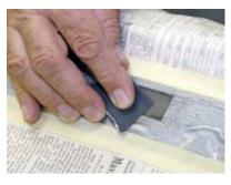
A putty knife was used to carefully scrape away the excess cement, and lightly wetted 400-grit sandpaper smoothed the surface. It's important that the cement is flush with the intake flange, as any recess can prevent the gasket from properly sealing. The identical procedure was performed on the opposite cylinder head and both were allowed to dry overnight.
