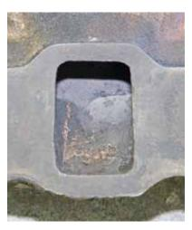
Through '71, the intake manifold's right-hand exhaust crossover passage is nearly double the size of the lefthand port. It was likely intended to reduce the amount of material located directly under the choke stove, providing optimal warm-up time. Exhaust leaks are common when combining a manifold of this vintage with later cylinder heads.
