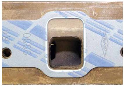
With a '71-and-earlier Fel-Pro intake manifold gasket in place, it's easy to see how the cement fills in the area that's otherwise missing. For the cost of a few dollars, this particular cylinder head is now compatible with any Pontiac intake manifold from '65 forward, as long as the correct intake gasket for the manifold is used.
