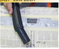
Once the cement was cement fully cured, it was checked for flatness using a straight edge—it was perfectly flat. Any high spots can be knocked down with sandpaper or a file if needed. A wet/dry vacuum was then employed to suck up all traces of dirt and debris before removing the tape and newspaper. Several passes were made to ensure that absolutely nothing would enter the engine. Even the slightest amount of grit can create significant internal damage.
